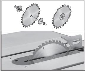
**Figure 36.** Order of blade component installation and teeth facing to the front.
